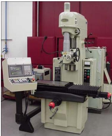
**Rebuilt Jig Borer with CNC Control.**
