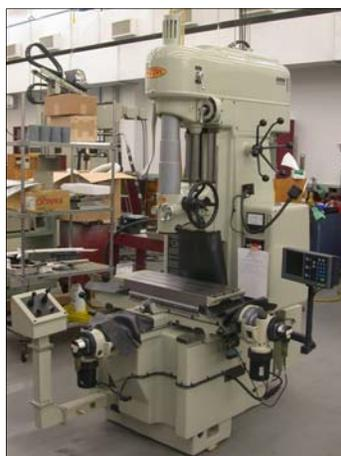
**Rebuilt Jig Borer with Digital Readout.**
