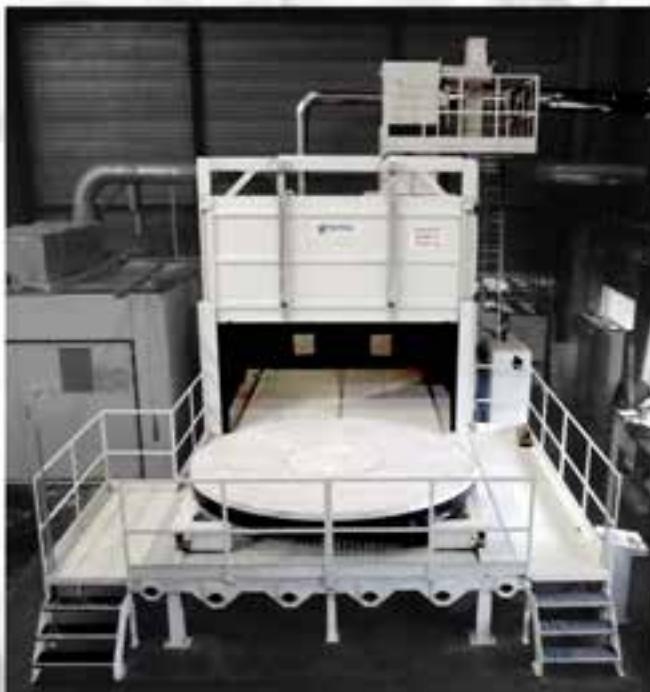
The shot blasting installation with mobile carriage is suitable for cleaning treatment of mergers or structures. The pieces are loaded on a turntable carriage designed for variable speed. To ease the operation, the loading of the heavy pieces on the carriage and their off-loading can be achieved by an overhead crane. The unit is composed of an airtight cabin where a series of turbines are applied to centrifuge the abrasive (steel shot) on the parts that slowly rotate.
